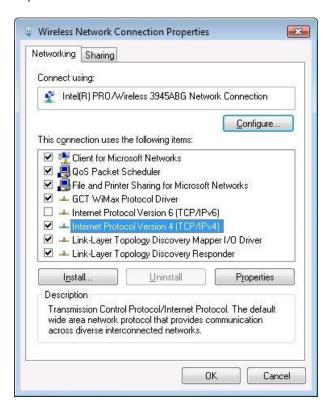
6. By default the router is going to have DHCP enabled, which means that if you select "Obtain an IP address automatically" and "Obtain DNS server address automatically", the router should lease you an IP and you should be ready to login.
