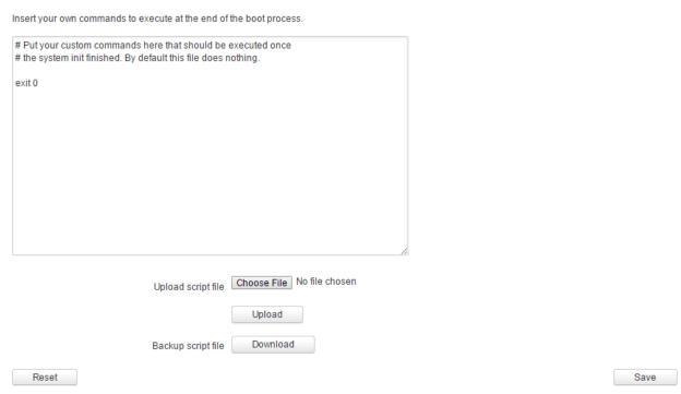
In *Script Management* window is shown content of a file /etc/rc.local. This file is executed at the end of startup, executing the line: sh /etc/rc.local In this script is needed to use sh (ash) commands. It should be noted, that this is embedded device and sh functionality is not full.
