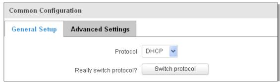
You can switch between Static, DHCP or PPPoE protocol by selecting the protocol that you want to use and then pressing **Switch Protocol**.
