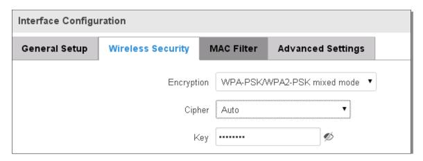
First select an encryption method: TKIP, CCMP, TKIP&CCMP and auto. Note: Some authentication methods won't support TKIP (and TKIP&CCMP) encryption. After you've selected your encryption method, you should enter your pass phrase, which must be at least 8 characters long.
