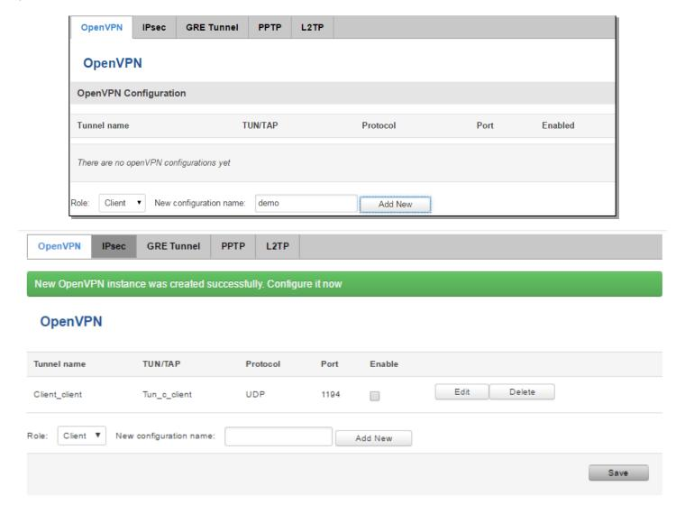
To see at specific configuration settings press "edit" button located in newly created configuration entry. A new page with detailed configuration appears, as shown in the picture below (TLS client example).
