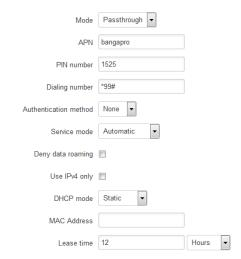
Using Passthrough Mode will disable most of the router capabilities!
