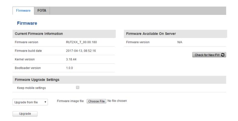
**Keep mobile settings** – if the check box is selected router will keep saved user mobile configuration settings after firmware upgrade.
