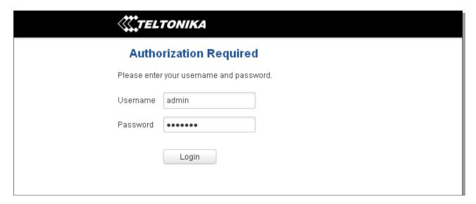
Enter the default password, which is "admin01" into the "Password" field and then either click Login with your mouse or press the Enter key. You have now successfully logged into the RUT230!
