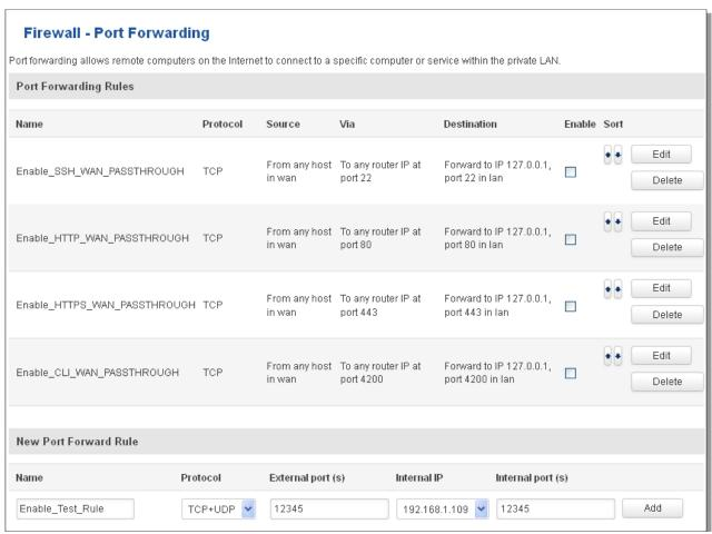
You can use port forwarding to set up servers and services on local LAN machines. The above picture shows how you can set up a rule that would allow a website that is being hosted on 192.168.1.109, to be reached from the outside by entering <a href="http://routersExternallp:12345/">http://routersExternallp:12345/</a>.
